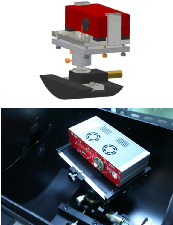
Fig. 11. Scheme of the PSAU-SiPM system mounted on stages (upper panel, 3D view of the rotary system; lower panel, photograph of the actual apparatus, showing the realized spot pointing at the detector surface).
